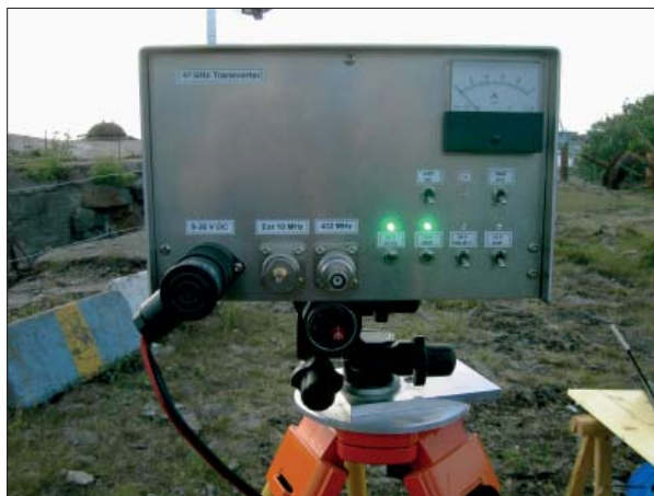
Transverter 47 GHz ready.
